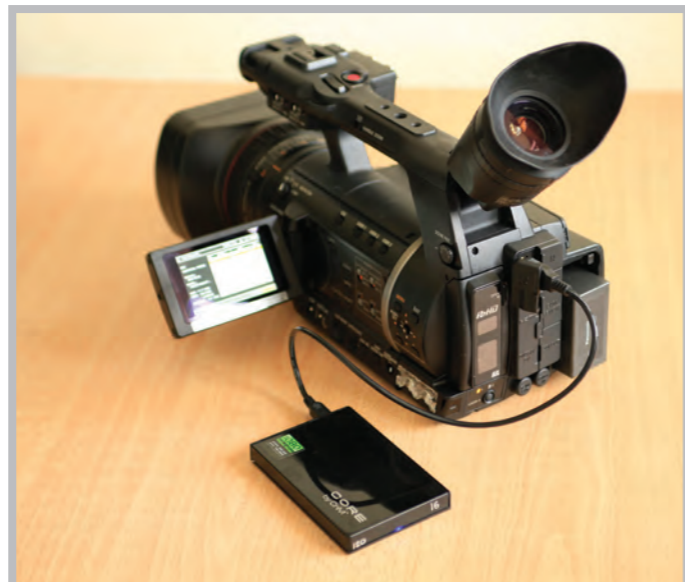
▲ A portable hard disk drive can be powered directly from the camera via the USB 2.0 port and the P2 cards can be backed up and verified
