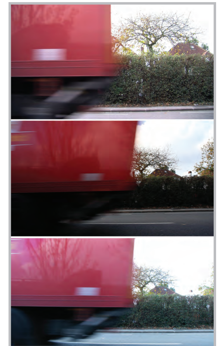
▲ CMOS sensors scan the image line by line, unlike CCDs which capture the whole picture in one go. When it comes to shooting moving objects this can result in 'skew'. Top: CCD sensor (JVC HM150); Middle: CMOS sensor (Canon 5D MkII); Bottom: MOS sensor (Panasonic HPX250). We can see that although the MOS sensor's rolling shutter still introduces some skew it is noticeably less than the CMOS sensor in the Canon 5D MkII
