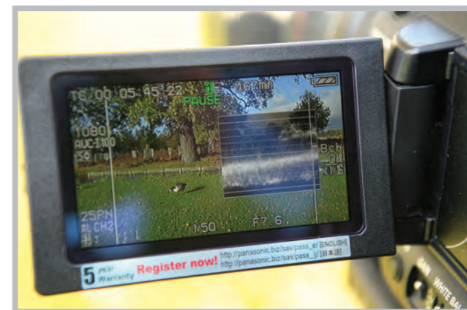
▲ The inclusion of a waveform monitor is just one of many professional features available on the AG-HPX250 EJ
